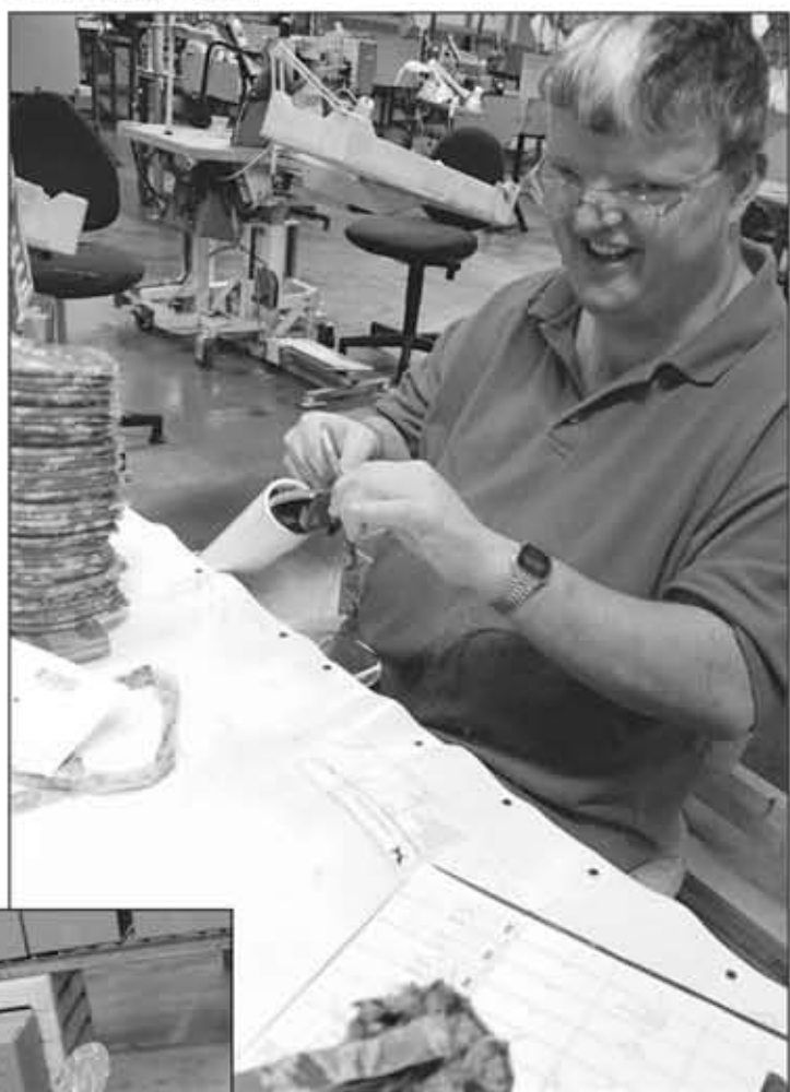
Donald Dozier (above) and Karl Stanton (left) have two different techniques for removing the excess thread from the military caps made by SEKRI. Stanton prefers scissors, while Dozier uses a mounted hair clipper to trim the stray threads.
